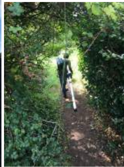
Electromagnetic conductivity imaging. This allows us to map the electrical properties of the shallow subsurface of the site, looking for evidence of buried structures and the natural (for example, hydrological) features of the site.
